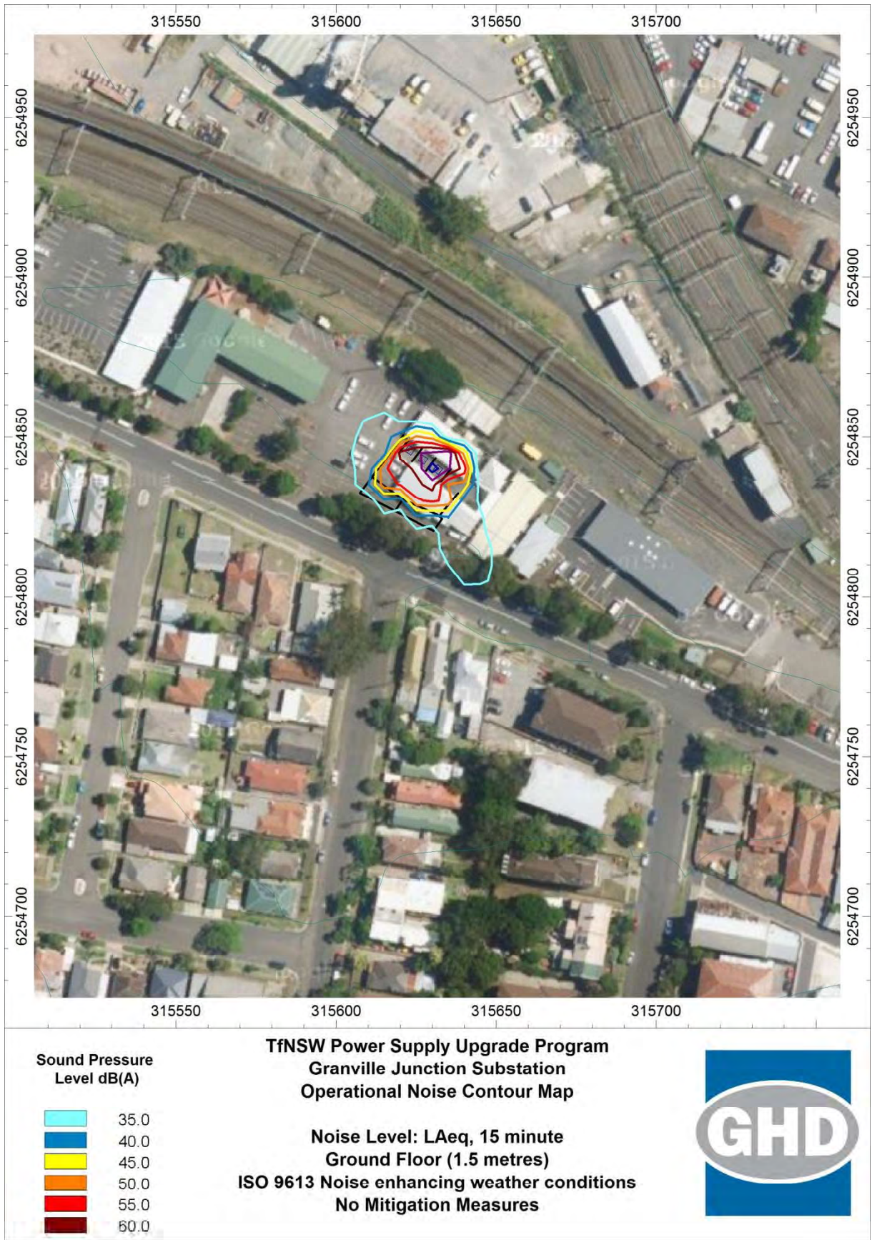
Figure 5-1 Case 1: Predicted L_{Aeq(night)} noise levels, dB(A) at a receiver height of 1.5 m
