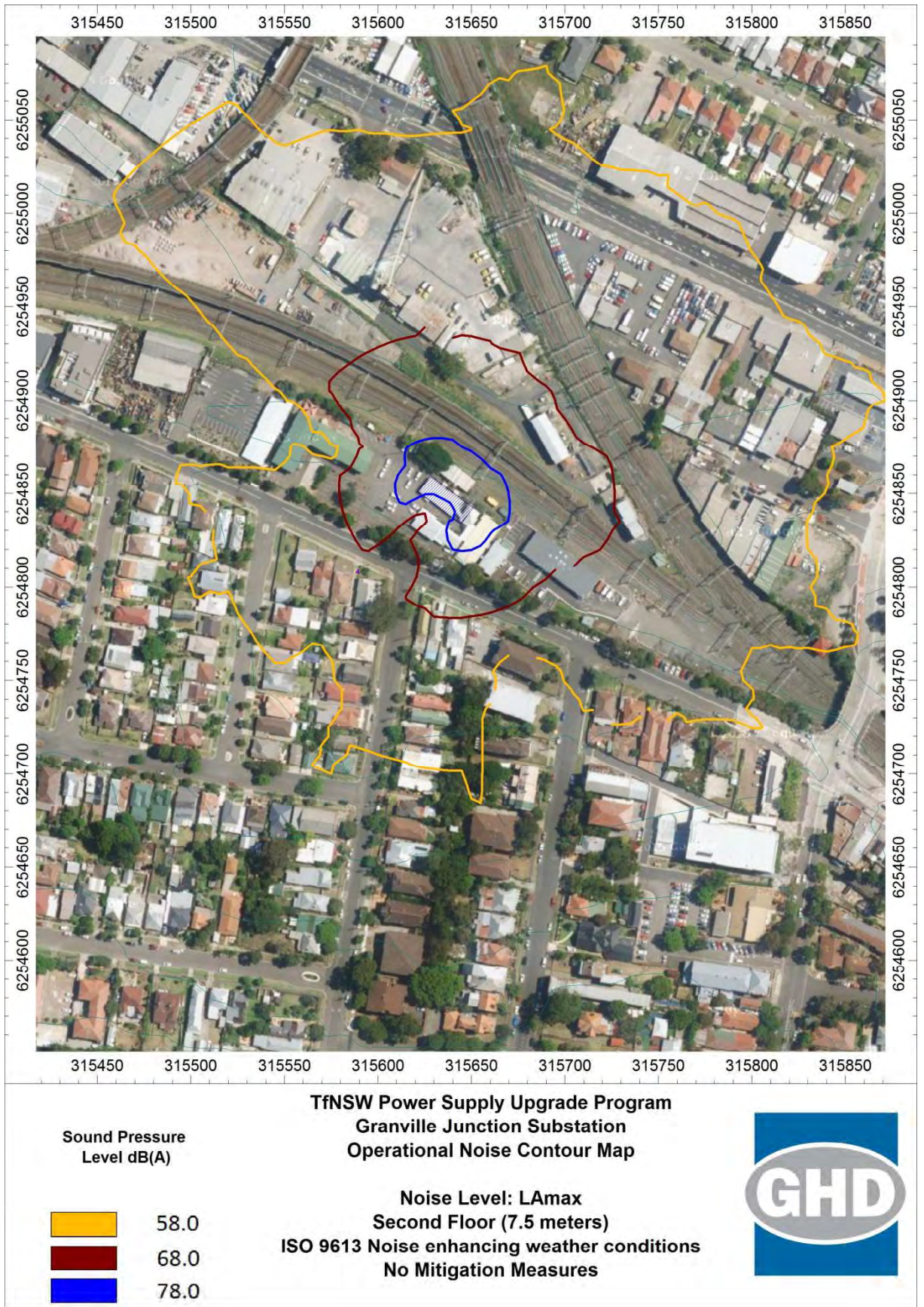
Figure 5-6 Scenario 2: Predicted L Amax noise levels, dB(A) at a receiver height of 7.5 m
