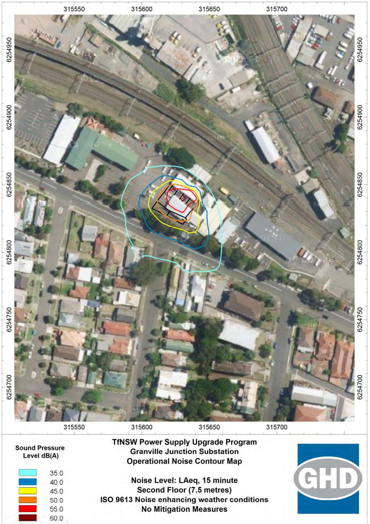
Figure 5-3 Scenario 1: Predicted L_{Aeq(night)} noise levels, dB(A) at a receiver height of 7.5 m
