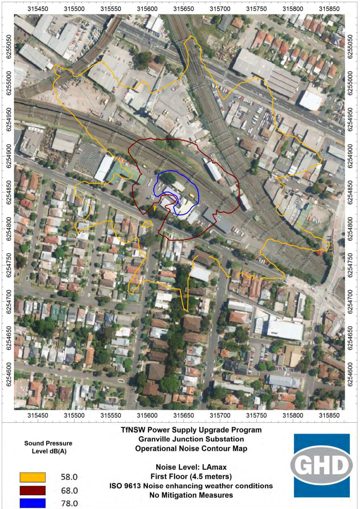
Figure 5-5 Scenario 2: Predicted L Amax noise levels, dB(A) at a receiver height of 4.5 m
